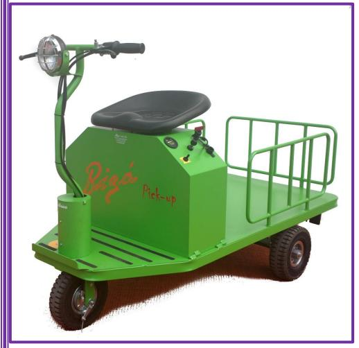
Small electric flatbed for transporting goods and for Picking on the ground. 151x74 with load plan cm. 95x74, autonomy 5 hours continuously, lead acid/gel batteries headlight, rear lights, horn, front drum brake, rear disc brake, parking brake, ignition key, ride on safety button, battery charge indicator, forward gear lever, neutral and reverse gear selection lever, quick external battery charger, lever for immediate disconnection of batteries, super elastic tires.
